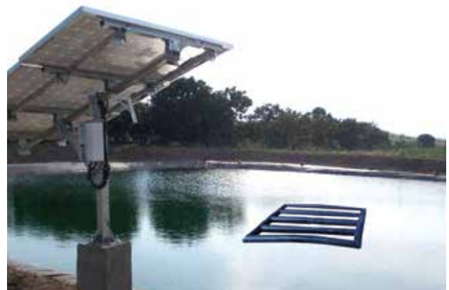
Jain Tarang (Floating) Platform in Farm Pond
