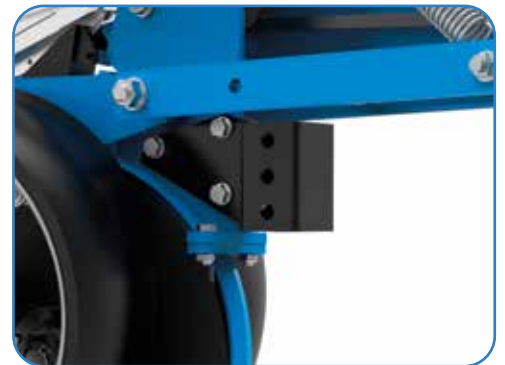
Optional : Mounting bracket for clod deflector or fixed row cleaner
