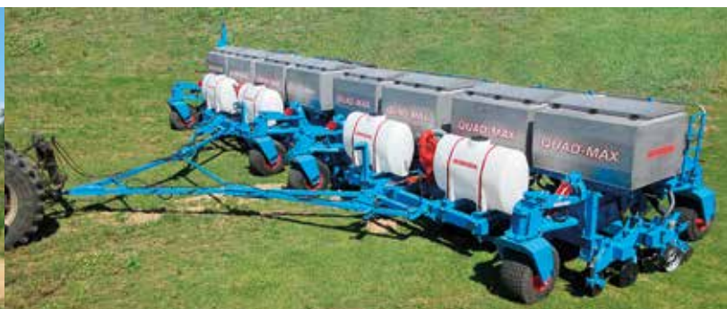
2 section QUAD-MAX type A in planting position
