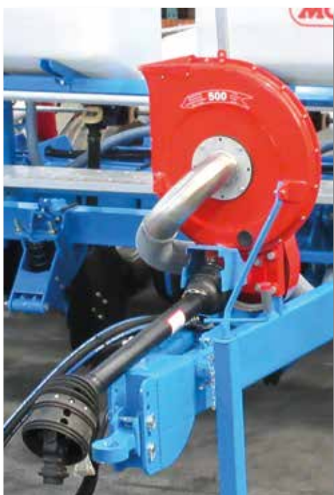
Standard drawbar with long wide-angle PTO shaft
