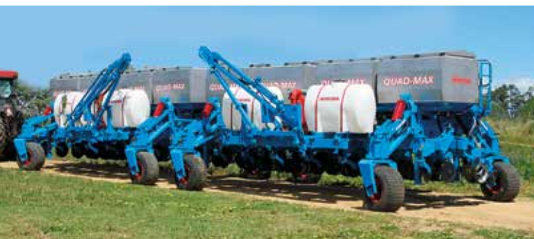
2 section QUAD-MAX type A in transport position
