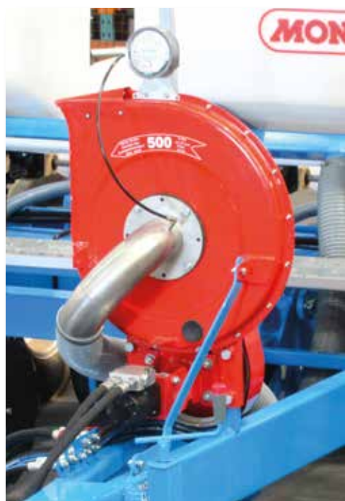
Optional hydraulic drive with vacuum gauge
